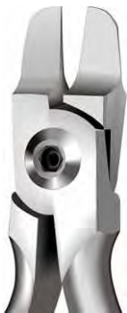
Tweed SI- 12-4611 T/C 11.5 cm/ 4½" Rectangular Arch Pliers, Tweed Style Forming plier for square or rectangular wires. The blades are designed to be parallel at .020" ( 0.51 mm) opening. The working edges are carefully diamond-honed to prevent wire scoring.
